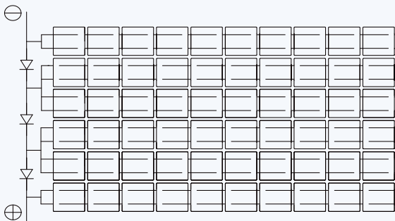
Figure 6: Electrical circuitry of cells and bypass diodes
